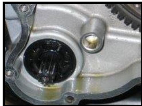
3) Wipe around the idler boss area with a clean rag to remove the excess oil, then use the surface cleaner cloth supplied to ensure the area is squeaky clean, ready for the JB Weld.
