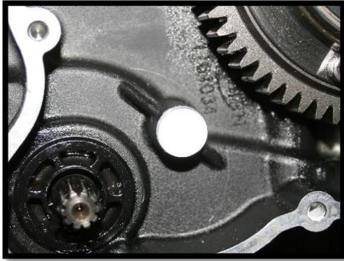
4) Stick the white dot supplied on to the idler boss to seal the hole. Squeeze an equal amount of JB Weld out of each tube on to a disposable surface (about 25% of each tube) and mix thoroughly.
