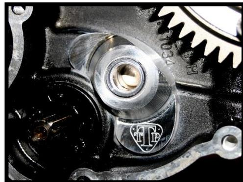
9) After 24 hours, the JB Weld will have cured and you can start reassembly.
