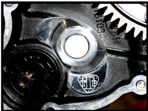
8) Wipe any excess JB Weld from around the edges of the Safe-Start and from the facing surface of the idler gear boss with a clean cloth. Use a clean part of the cloth for each wipe or it'll just keep smudging. Now remove the white sticky dot from the top of the boss.
