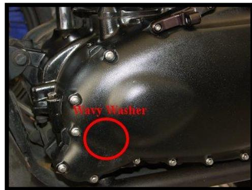
Don't lose the wavy washer which is located behind the clutch cover.
