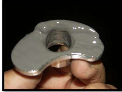
5) Now put on the glove supplied and apply a thin layer of JB Weld to the idler boss. Ensure JB Weld is worked in to the grooves in the tower and then completely cover the bottom of the Safe-Start as shown.
