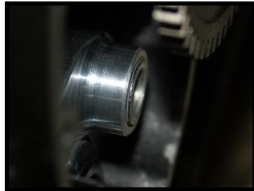
7) Keep pressure on the Safe-Start until the top of the idler boss protrudes slightly from the top of the Safe-Start.
