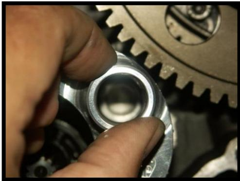
6) Look through the hole in the Safe-Start to centralize the idler boss before pushing the Safe-Start home.
